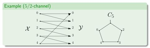
The zero-error capacity C(G) with L = 1 only depends on G.
