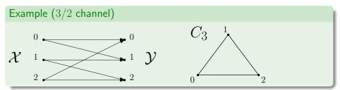
It can be seen that  $C(C_3) = 0$ . A code that achieves zero-error with list of size 2 for this channel is known as 3-hash code or trifferent code.
