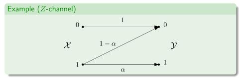
We note that  $(x, y) \in E$  if and only if y can be received at the channel output when x is transmitted over the channel.
