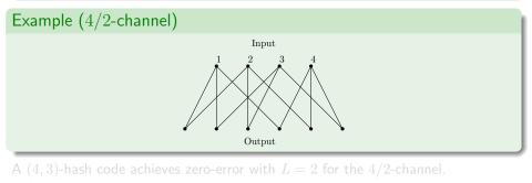
Zero-error capacity for L < k - 1 is 0 while for L = k - 1 is positive.
