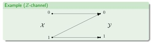
We note that  $(x, y) \in E$  if and only if y can be received at the channel output when x is transmitted over the channel.
